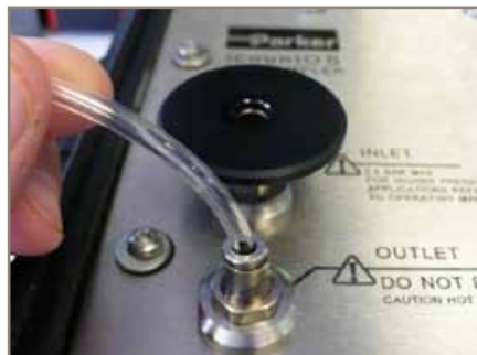
Attach OUTLET (Ø 4mm) hose
