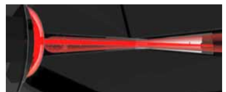
Fig 3. A cast image or shadow created by the contaminant in the oil creates a measurable change in the light intensity.
